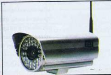
The camera has a built-in web server which allows users to control it remotely via browsers.
